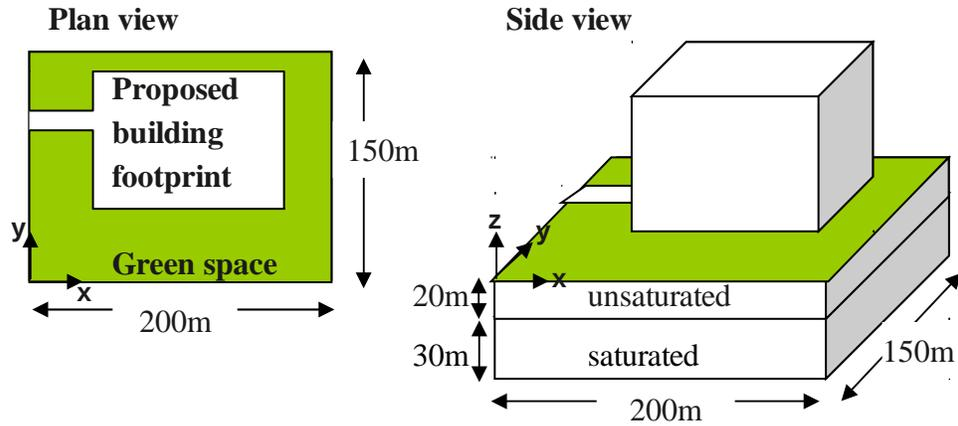
Engineers are estimating the area of green space needed for a new housing development to meet NYC's policy to increase infiltration and reduce runoff.
